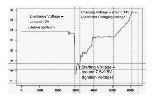
•Discharge Voltage: When the ignition OFF, engine OFF (Over 20 Minutes), the Discharge Voltage should be around 12V. If the discharge voltage is lower than 11V, it will be hard to turn the ignition ON. If the discharge voltage continuously stay under 11V, it means the battery is aging and replacement is needed.
